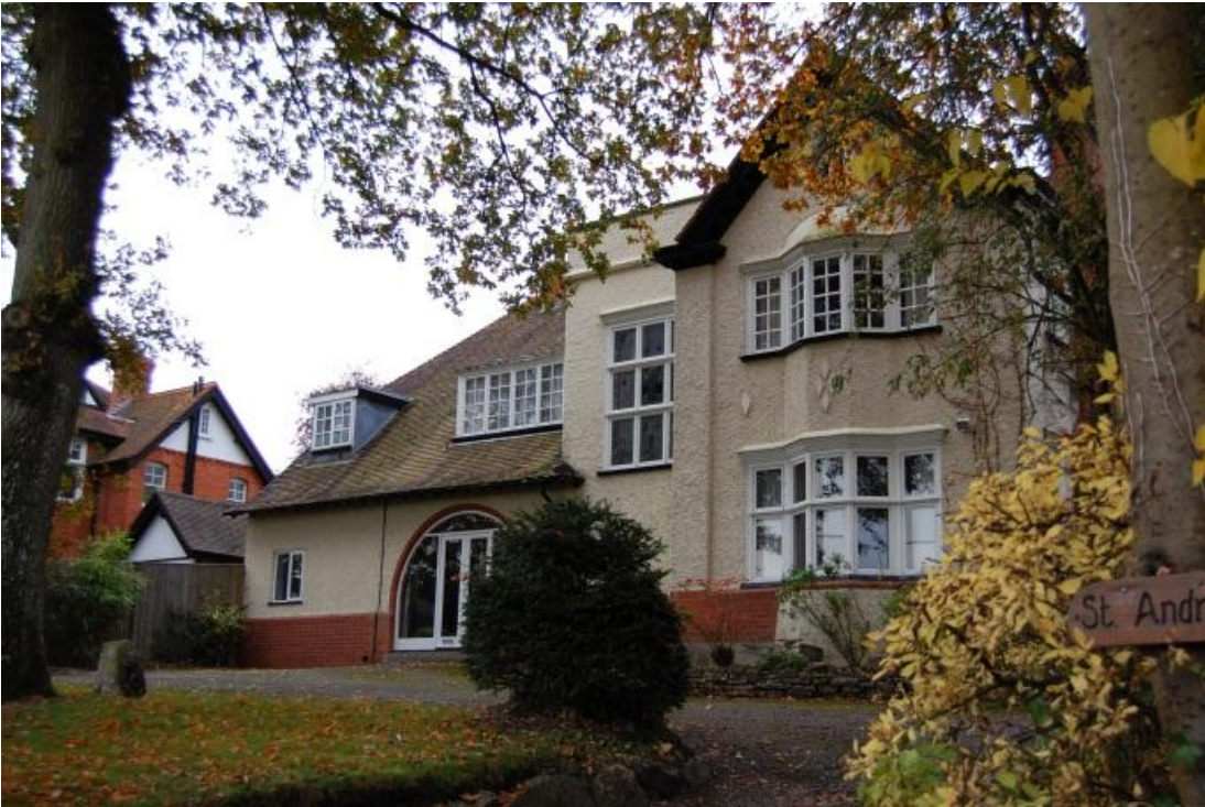
St. Andrews, a good example of Edwardian housing with strong references to the Arts and Crafts movement particularly with regard to the bay and stair windows.
