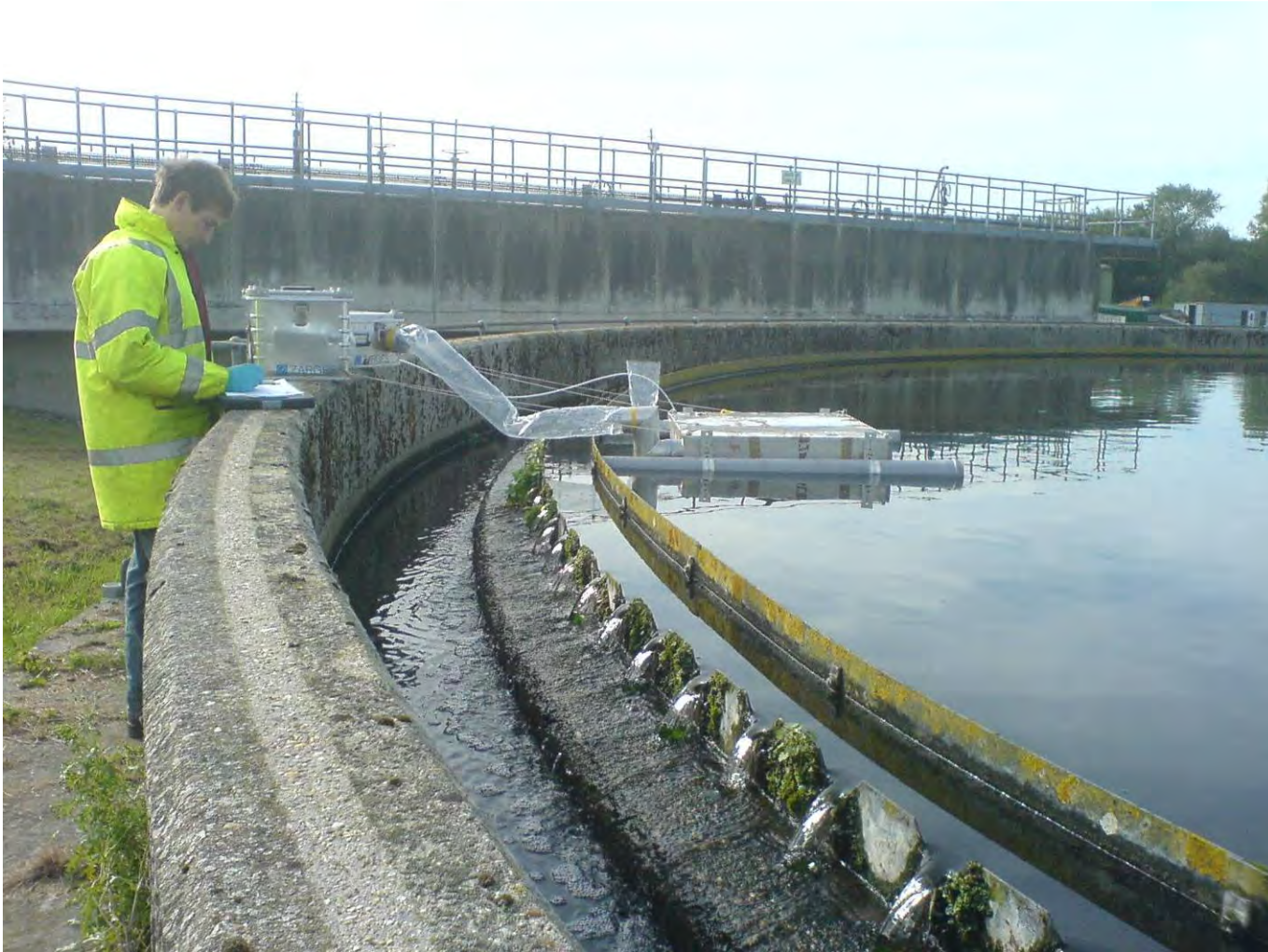
Fig 2, The Lindvall type hood collecting surface emissions (on another site) from a settling tank, fan and filter on the wall the 1m 2 hood connected with Nalophan NA tube
