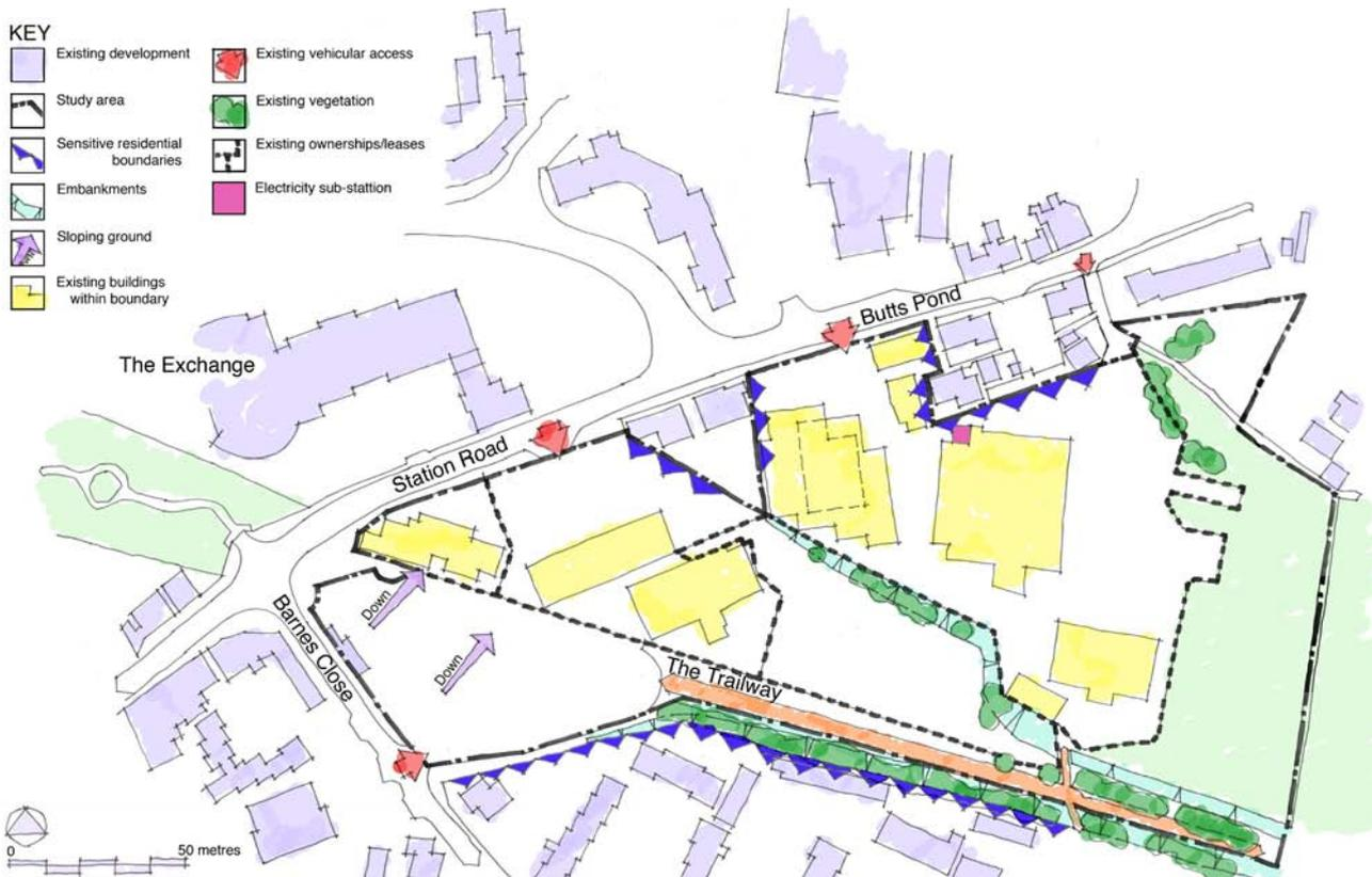
Figure 22: Site constraints plan
