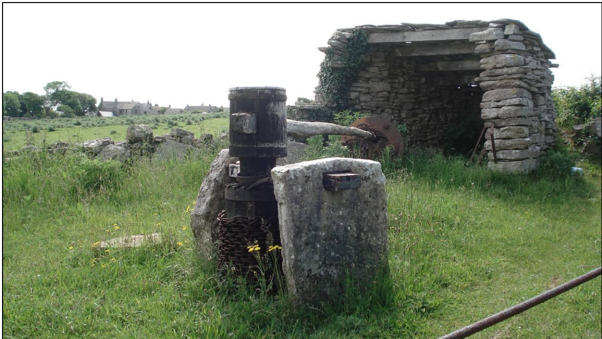
FIG. 2: Norman's Quarry. The spack, capsten, sheds and shaft of a former stone quarry preserved by the National Trust at Castle View.
