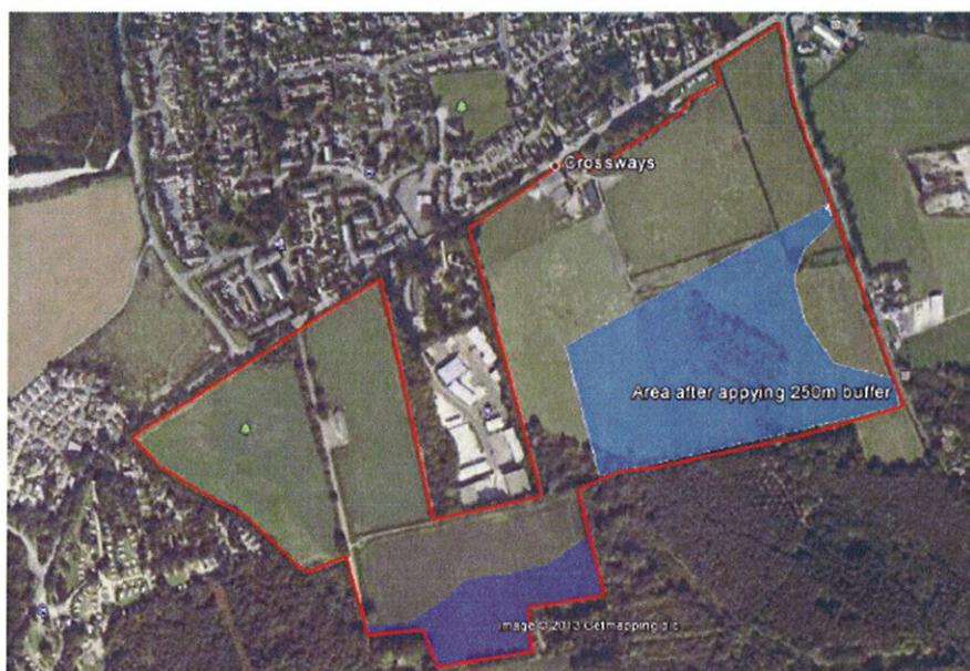
Figure 4: Area potentially available for quarrying after applying 250m buffer to Crossways Village and particularly sensitive receptors
